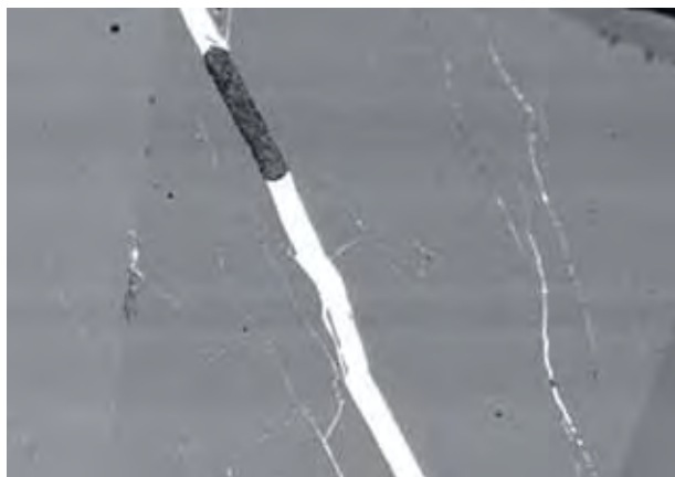
Figure 17. This back-scattered-electron image (taken with a scanning electron microscope) shows lead glass-filled fractures of varying widths. Because of the higher average mass of elements in the glass, it is much brighter than the host ruby. Width of the image is about 1.6 mm.
