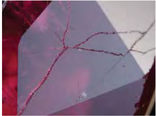
Figure 22. At 800°C, the lead-glass filler actually started to bubble where fractures reached the surface. Photomicrograph by C. P. Smith; magnified 22×.
